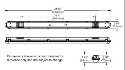
Power Consumption: 65W Current: 0.54 – 0.23 amps Input Voltage: 120 - 277VAC
