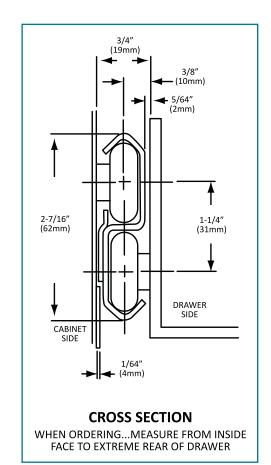
NOTE: STAINLESS STEEL BALL BEARING ASSEMBLIES W/REMOVABLE STAINLESS STEEL THREADED FASTENERS (MODEL NO. 552-X001) AND DELRIN BEARING COMPLETE W/REMOVABLE STAINLESS STEEL THREADED FASTENERS (MODEL NO. 552-X101) MAY BE ORDERED SEPARATELY...SEE PAGE G30
